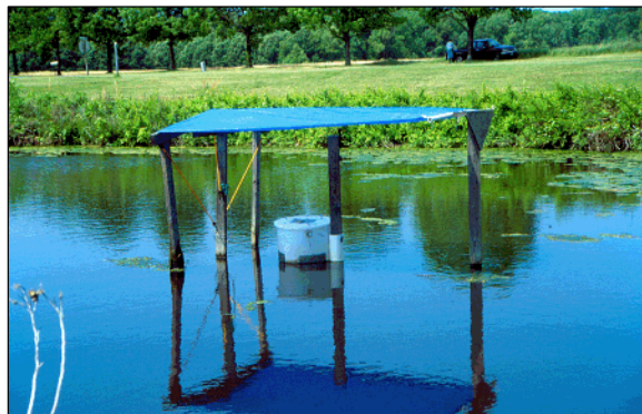
Figure 4. Small fish deployment cages; (a) protective barrel and smaller floating baskets; (b) deployed barrel with lid removed to reveal arrangement of floating baskets; (c) fish cage deployed in the Research Pond at University of Maryland - Wye Research and Education Center with blue tarp to provide shade.
